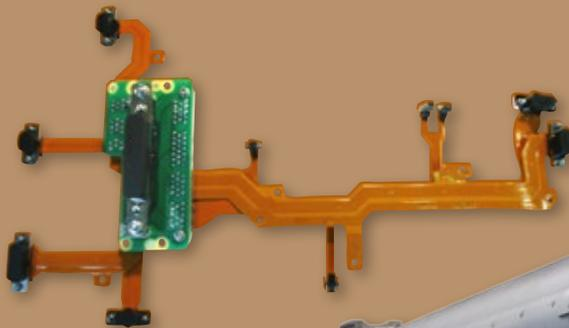
A single, integrated, multi-branch flex circuit assembly is orders of magnitude smaller and lighter than an equivalent ribbon cable or discrete wire harness. Well-conceived flex circuit designs can efficiently replace bulkier hard printed circuit boards, heavier
