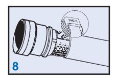
IMPORTANT: Always roll band through the buckle slot twice (see Step 3). Bands must be double-coiled to function correctly. The failure to roll the band through the buckle slot twice is the most common user error in band style terminations.
