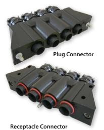
Available with three, four and six contacts, typical for traction motor applications. Suitable for single cables AWG 4 – 373MCM (35 to 185 mmg). Working voltage up to 3000 Vcc.
