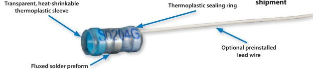
AS83519 TYPE • 81824/1 QUALIFIED Heat Shrink Termination Sleeves and Mil-Qualified In-Line Splices
