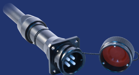
SUPER ITS-IFO B FIBER OPTIC CONNECTORS 4-Pole fiber optic, shell size 16S connector with environmental sealing strain relief backshell and Kevlar fiber retention
