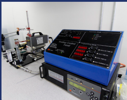
Brazing control panel
