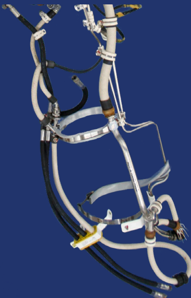
Metal-core conduit wire protection aircraft brake assembly
