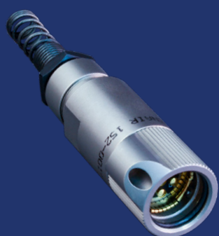
Audio plug, field serviceable, with wire strain relief and rigid contacts, crimp and solder cup
