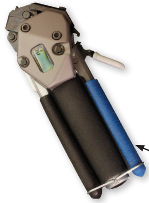
Color-coded tensioning lever: blue = micro
