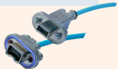
Plug with male MT ferrule and retaining plate
