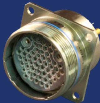
MIL-DTL-83723 type filter connector, gold-plated for atomic oxygen corrosion resistance
