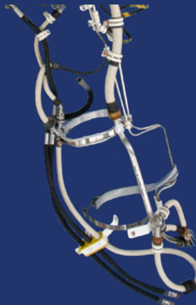
Metal-core conduit wire protection aircraft brake assembly
