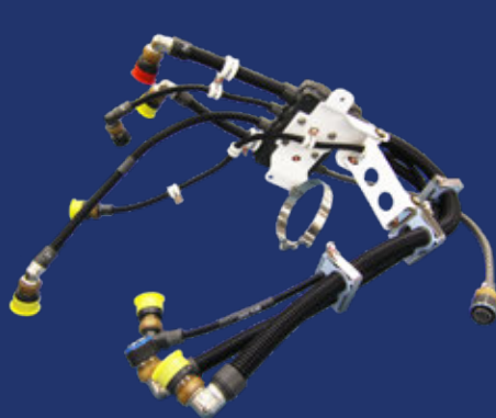
Complex multibranch fighter jet electrical wire conduit assembly
