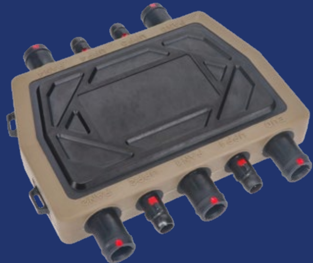
STAR-PAN NG 4/4 P/N TS2-014 Next-generation design with one EUD port, four pan ports and four universal power ports
