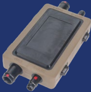
STAR-PAN NG 1/2 P/N TS2-011 Our smallest hub with one EUD port, one pan port and two universal power ports
