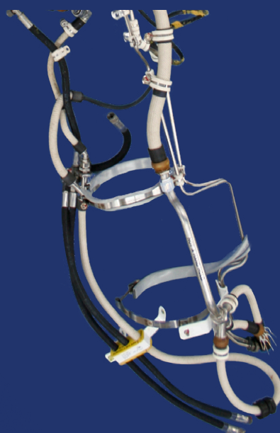
Metal-core conduit wire protection aircraft brake assembly
