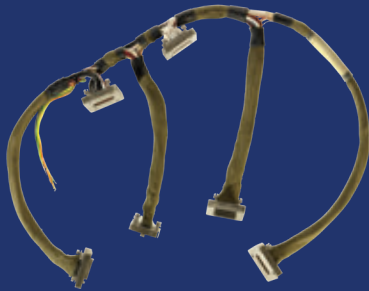
Multibranch wire harness with Glenair Micro-D connectors
