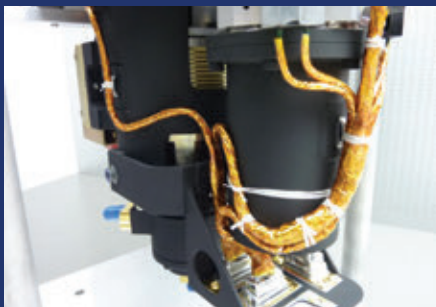
Harness integration into space payload electromechanical devices
