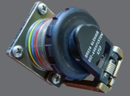
Full environmental threaded / twist-lock seal
