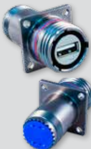
233-345 E-42 SuperSeal Connectors with Accessory Threads and USB 2.0 Male (Plug) or Female (Receptacle) Interface to Crimp Removable Contacts
