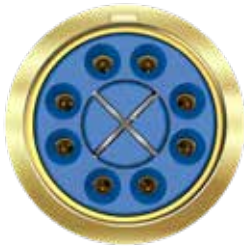
Ochoito "Blue" for SuperSpeed USB Pin contact mating face
