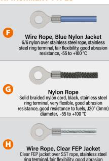
Clear FEP jacket over SST rope, stainless stee ring terminal, fair flexibility, good abrasion resistance, 100" diameter, -55 to +200 °C
