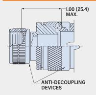
For Profile M and M 45° and 90° backshells, the length increases by 1 inch.
