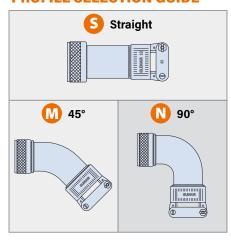
Shielded. Straight, 45° or 90°. 380P\*105 backshell fits Glenair Series 970 PowerTrip connectors. Spin coupling, non-environmental. For use with shielded cable. Type H heavy duty saddle clamp has stainless steel telescoping fillister head screws and lockwashers. Two ground rings for terminating both individual and overall braid shields. Anti-decoupling mechanism provides audible detented coupling and prevents backoff under high vibration. Available in aluminum or stainless steel.
