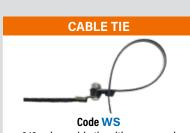
6/6 nylon cable tie with screw and locknut. 1.77 (45.0) max. wire bundle dia. -40 to +85 °C.
