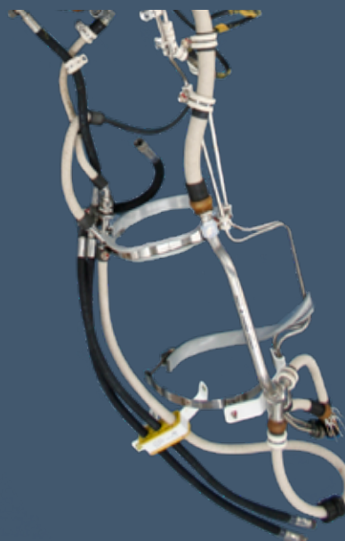
Metal-core conduit wire protection aircraft brake assembly
