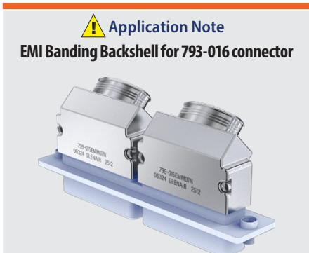
Use backshell part number 799-015 (Size M). Two backshells are required per connector. Two piece backshell has lip to lock into groove on connector. Available in top entry, side entry and 45° entry.
