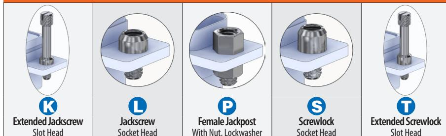
Screwlocks allow connector to be plugged in before the screws are tightened. Jackscrews must be tightened in order to mate connector.
