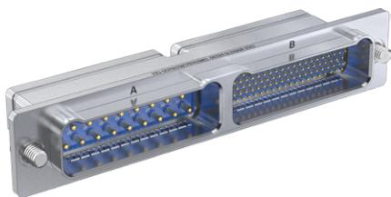
**Dual bay cable mount.** Space-saving 793-017 connector features high-density, high current and high frequency capabilities, saves size and weight compared to legacy rack-and-panel types. Connector has two inserts. Machined scoop-proof shell has groove for attaching backshell. Size 23 contacts are included with connector; size 8, 12, and 16 contacts are ordered separately. Connectors become non-scoop proof at parallel horizontal angles of entry from 16°–47°.
