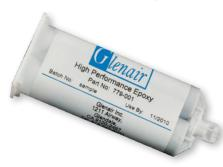
High performance flexible two part thermoset epoxy provides high strength flexible bond from -75 °C to 150 °C. 50 ml duo syringe fits standard dispensing guns. Use with square green mixing nozzle sold separately. 12 hour cure time at 20 °C, 1 hour at 85 °C, 30 minutes at 150 °C. Apply to inside of boot with wooden spatula. 18 month shelf life.
