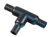
Low profile "Tee" heat shrink transitions provide an easy to install and rugged cable routing solution. Transitional boots are available in eight material options with five adhesive choices. All Adhesive lined and unlined shrink books are RoHS compliant. Transitional boots are water-tight when equipped with factory installed or user-installed adhesive. Choose boot size based on cable diameter.
