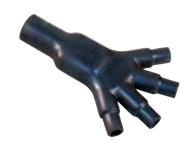
1:4 wide body, heat shrink transitions provide an easy to install and rugged cable routing solution. Transitional boots are available in eight material options with five adhesive choices. All adhesive lined and unlined shrink books are RoHS compliant. Transitional boots are water-tight when equipped with factory installed or user-installed adhesive. Choose boot size based on cable diameter.
