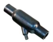
30° angle "Tee" transition heat shrink boots provide an easy to install and rugged cable routing solution. Transitional boots are available in eight material options with five adhesive choices. All adhesive lined and unlined shrink books are RoHS compliant. Transitional boots are water-tight when equipped with factory installed or user-installed adhesive. Choose boot size based on cable diameter.
