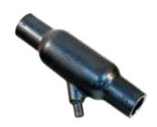
45° angle "Tee" transition heat shrink boots provide an easy to install and rugged cable routing solution. Transitional boots are available in eight material options with five adhesive choices. All adhesive lined and unlined shrink books are RoHS compliant. Transitional boots are water-tight when equipped with factory installed or user-installed adhesive. Choose boot size based on cable diameter.
