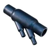
Double angled "Tee" transition heat shrink boots provide an easy to install and rugged cable routing solution. Transitional boots are available in eight material options with five adhesive choices. All adhesive lined and unlined shrink books are RoHS compliant. Transitional boots are water-tight when equipped with factory installed or user-installed adhesive. Choose boot size based on cable diameter.
