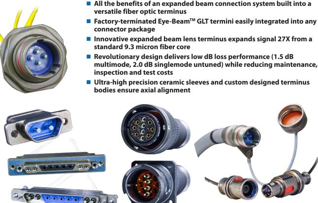
Eye-Beam<sup>™</sup> GLT Expanded Beam fiber optic termini can be integrated into virtually any circular or rectangular connector package. Factory terminated lens pin termini and lens socket termini on cable jumpers allow for easy fusion splicing in the field.
