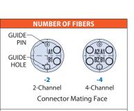
There is a rotational relationship between D-flat on the panel cutout and the jam nut receptacle connector mating face.
