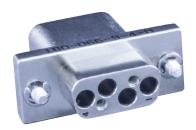
Micro-D form-factor GFR Socket Plug. Supports from one to eight GFR socket termini with insertion loss performance comparable to industry-standard MIL-PRF-29504. Precision-machined with integral alignment pin holes for optimum optical fiber alignment and low dB data loss performance. Available in aluminum and stainless steel. Termini sold separately. Supports single- and dual-O-ring termini.
