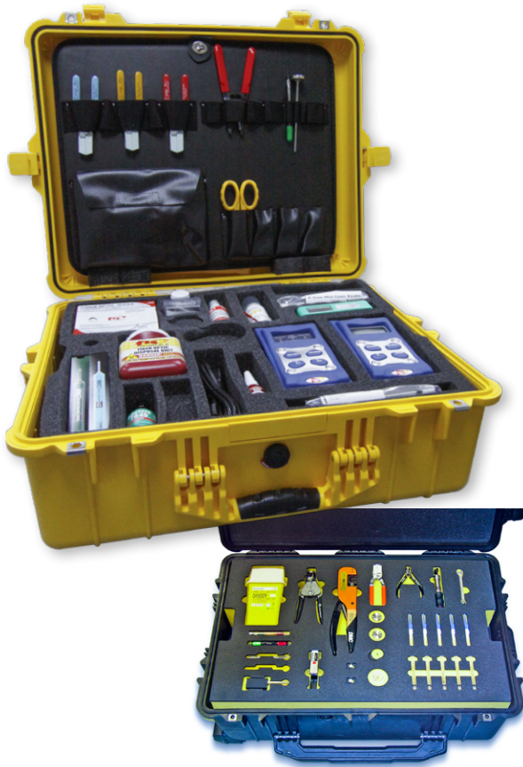
Glenair Fiber Optic Toolkits contains all of the tools you will need for fiber optic termination, plus a laminated card with termination instructions.
