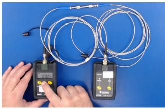
2. Insert probes into calibration adapters. Tactile click will be felt when properly seated.
