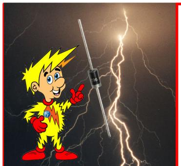
Designers must protect systems from transient overvoltages as a result of nearby lightning strikes. Placing transient suppression diodes within the system preferably inside a connector instead of some ad hoc location—is one of the most effective ways to protect electronic systems from lightning strikes and other sources of electromagnetic pulse.
