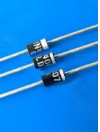
Diode power is rated in watts for a given pulse shape and pulse duration. Typically the reference values are given for a  $10/1000\mu$ s pulse. This means that the diode can absorb the peak power rated for a pulse with  $10\mu$ s rise time and  $1000\mu$ s fall time. If the system is subjected to a different pulse shape or duration the value must be adjusted accordingly. The table on the following page does just that for RTCA D0160 lightning strike.
