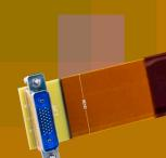
Rigid flex point-to-point jumper with Series 79 Micro-Crimp connectors and a small form-factor hybrid fiber optic tool segment connector
