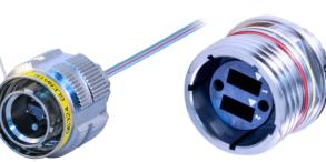
Plug with EMI/RFI ground spring Shell size-insert arrangement 11-1, Up to 24 fibers (1 MT ferrule)
