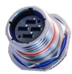
Jam nut receptacle Shell size-insert arrangement 17-4, Up to 96 fibers (4 MT ferrules)
