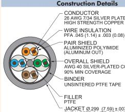
26 AWG 7/34 SILVER PLATED HIGH STRENGTH COPPER ALLOY WIRE INSULATION
