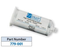
High performance flexible two part thermoset epoxy provides high strength flexible bond from -55° to 150°C. 50 mL duo syringe fits standard dispensing guns. Use with square green mixing nozzle sold separately. 12 hour cure time at 20°C, 1 hour at 85°C, 30 minutes at 150°C. Apply to inside of boot with wooden spatula. 18 month shelf life.
