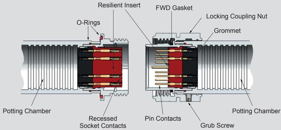
Receptacle (left) and Plug (right) connector pair
