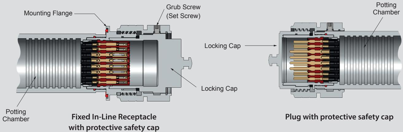
Fixed In-Line Receptacle with protective safety cap
