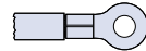
Small Ring for Attaching Receptacle Covers to a Panel with a Screw
