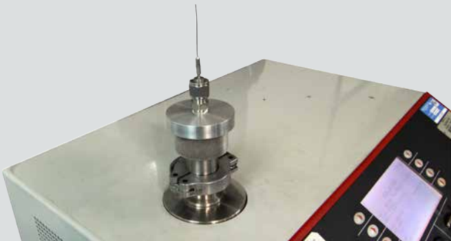
Close up of gas tube assembly undergoing helium leak test at the Glenair Factory in Glendale, CA
