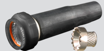
317V111 Piggyback Boot Adapter These composite, self-locking backshells have a drop-in banding adapter and are supplied with pre-attached shrink boot Page 173
