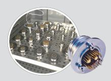
Connectors utilizing CODE RED hermetic encapsulant sealing went through a grueling qualification test and validation process to prove material durability and hermeticity. Validation testing including 100 cycles of thermal shock IAW EIA-364-32 Test Condition A -65°C to +200°C while maintaining hermeticity followed by 1000 hours of thermal aging at 200°C. Additional tests included:
