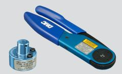
809-127 (M22520/4-01) crimper for use with size #16 coax Series 806 contacts. Requires positioner, ordered separately. These crimp tools perform precision eight indent crimps for wire terminations and excellent tensile strength. Ratchet mechanism prevents improper crimps. Use with bayonet-type positioners. Length is 9.75 inches, weight is 15 oz.
