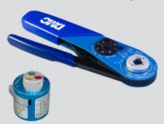
809-136 (M22520/1-01) crimper for use with size #12, and #16 Series 806 contacts. Requires positioner, sold separately. These crimp tools perform precision eight indent crimps for wire terminations and excellent tensile strength. Adjustment wheel has 8 settings for wire being used. Ratchet mechanism prevents improper crimps. Use with bayonet-type positioners. Length is 9.75 inches, weight is 15 oz.
