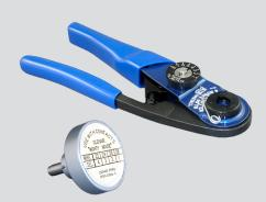
809-015 (M22520/2-01) crimper for use with size #20HD and #22HD signal contacts and #8, #12, #16 co-axial and tri-axial Series 806 contacts. Requires positioner, sold separately. These crimp tools perform precision eight indent crimps for wire terminations and excellent tensile strength. Adjustment wheel has 8 settings. Ratchet mechanism prevents improper crimps. Use with bayonet-type positioners. Length is 6.75 inches, weight is approx. 10 oz.
