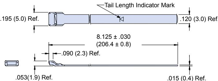
**The 600-057 Micro Band** is precision constructed of 300 Series SST/Passivate, and designed for use with the 600-061 Hand Banding Tool or the 600-068 Pneumatic Banding Tool. Double-wrapped bands will accommodate diameters up to approximately .88 inches (22.4). Bands may be ordered flat (600-057), or precoiled (600-057-1). Bands come bagged and tagged in quantities from 1 to 100.
