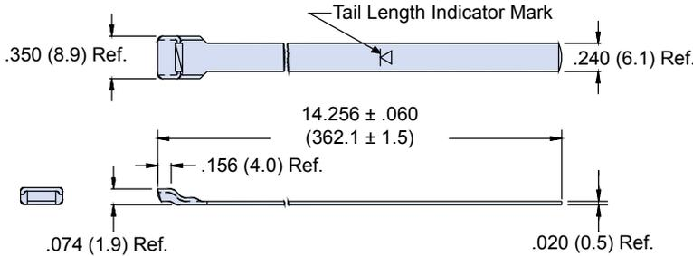
**The 600-052 Standard Band** is precision constructed of 300 Series SST/Passivate and designed for use with the 600-058 Hand Banding Tool or the 600-067 Pneumatic Banding Tool. Double-wrapped bands will accommodate diameters up to approximately 1.8 inches (45.7). Bands may be ordered flat (600-052) or precoiled (600-052-1). Bands come bagged and tagged in quantities from 1 to 100.
