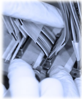
Potting a Micro-D with Epoxy-Filled Syringe
