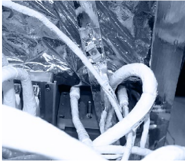
Detail of the Atmospheric Infrared Sounder Instrument (AIRS) with Glenair Micro-D Cables and Connectors Photo courtesy JPL
