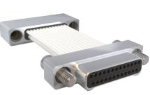
Glenair Back-To-Back Cable Assemblies are offered in three configurations and feature gold alloy TwistPin contacts. Contacts are precisioncrimped to insulated, stranded wire. These nanominiature connectors offer premium performance and reliability for demanding applications. Contact rating, DWV rating 250 volts AC. Wire gages #30 and #32 AWG. Connectors are wired 1 to 1, 2 to 2, 3 to 3 etc.
