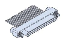
Glenair Uninsulated Wire Nano Connectors feature gold alloy TwistPin contacts. Contacts are precision-crimped to solid wire. These nanomimiature connectors offer premium performance and reliability for demanding applications. Contact spacing is .025 inches. 1 amp current rating, DWV rating 250 volts AC. Wire gages #30 and #32 AWG.
