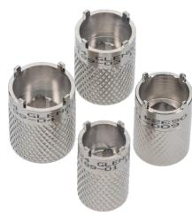
**1/4" Socket Drive** for use with rear panel mount receptacle mounting nut. Alloy steel construction and nickel plated. Order by insert arrangement individually or in a kit
