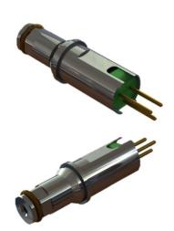
Size 8 Cavity Opto-electronic contacts transmit and receive TTL/CMOS compatible electrical signals over Multimode fiber optic cable. Transmitters consist of a laser driver and an 850nm VCSEL laser. Receivers consist of an 850nm PIN Photo Detector and an Amplifier. Output data signal is TTL/CMOS compatible.
