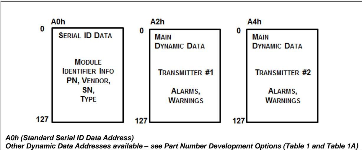
The PCB mount Dual-Transmitter features EEPROM for Serial ID, which contains the product data stored for retrieval by host equipment. This data is accessed via the 2-wire serial EEPROM protocol derived from with the industry standard SFP Multi-Source Agreement but modified to account for Dual-Transmitter functionality. The base EEPROM memory, bytes 0-255 at memory address A0h, is organized in compliance with SFF-8074i.
