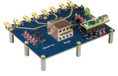
The 050-334-EVALBOARD can be used to evaluate 050-333 Board Mount Dual Optical Transceiver Operating from 100Mbps to 5Gbps data rate. The transceivers can be used for bidirectional fiber optic link over 4 multimode  $50\mu m/125\mu m$  or  $62.5\mu m/125\mu m$  type fiber optic cables.
